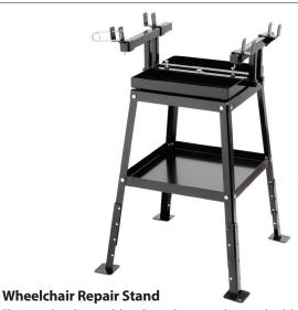
Eliminate bending and kneeling when completing wheelchair repairs with this convenient stand. Simply attach the wheelchair frame to the top of the stand using the included pins. It accommodates most 14" – 22" wide chairs with  $\frac{7}{8}$ " or 1" tubing and features adjustable height, 360° top rotation and built-in tool shelf.
