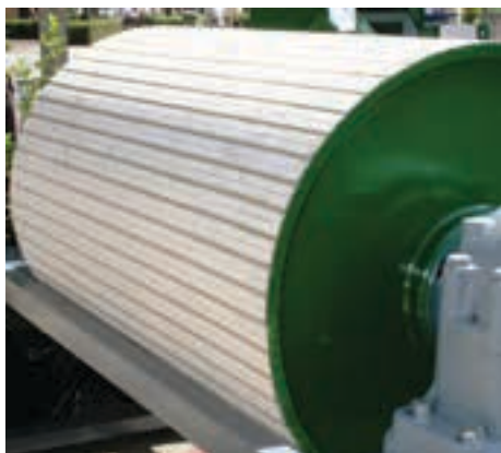
MultoLag™ pulley lagging functions as a maintenance-free, wear-resistant cover that is applied to pulley shells to improve traction in the case of drive pulleys and provide a polished low friction surface on non-drive pulleys.
