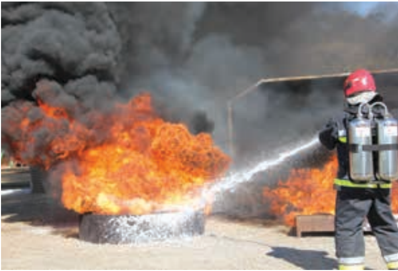
The Backpack water mist system being used on a fuel spill fire. The environmentally friendly system rapidly extinguishes 250 litres of burning fuel using 12 litres of water. According to ASP Fire, this has the same knock out power as a 500 litre trailer-mounted system.
