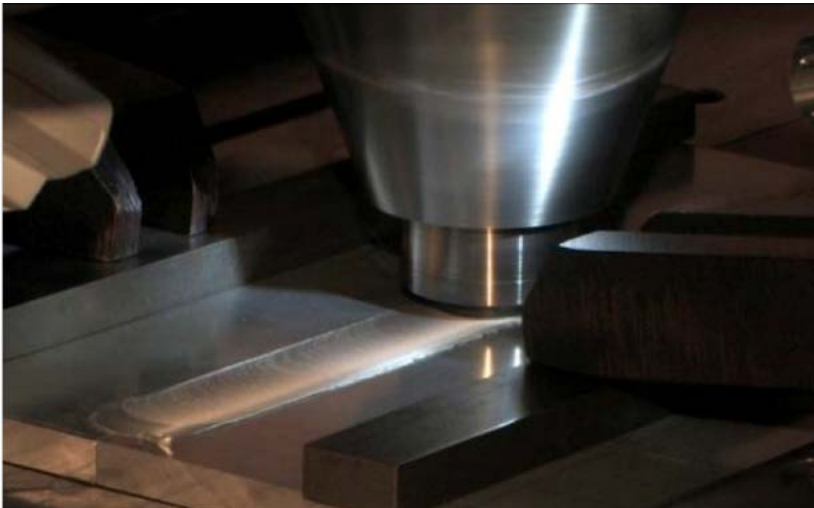
Friction stir welding invented by Wayne Thomas of TWI
