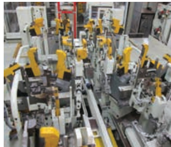
Above: A pneumatic clamping system used in an automotive assembly plant. In South Africa SMC's biggest market is for the Car Project (CP) range, which includes automotive solutions for passenger and commercial vehicle production.
