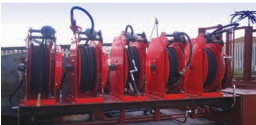
Heavy-duty retractable reels are used for high performance transfer of lubricants and abrasive fluids.
