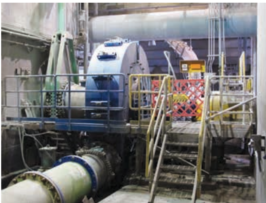
KSB Pumps and Valves' MDX 750c. MDX extra-heavy mill duty pumps are the heart of mill circuits, tackling the most extreme duty conditions.
