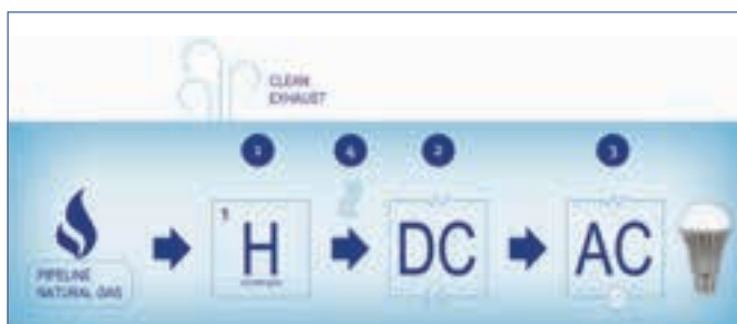
Above: The PureCell is designed to be powered by natural gas rather than hydrogen. The gas ( CH_4 ) is ‘cracked’ to provide the hydrogen needed to fuel the cell. Right: Doosan fuel cells use phosphoric acid ( H_3PO_4 ) as the electrolyte, saturated in a silicon carbide matrix (SiC). The electrodes are made of carbon paper coated with a finely dispersed platinum catalyst.
