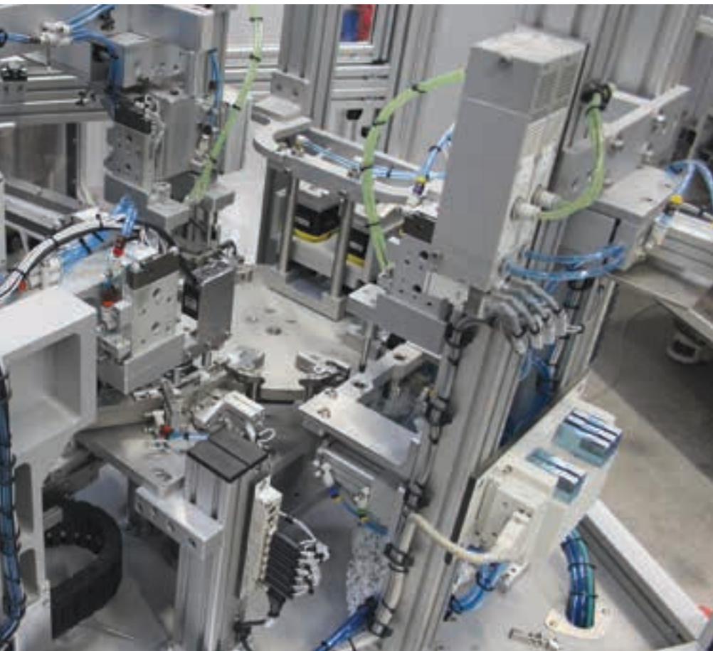
Above: A pneumatic clamping system used in an automotive assembly plant. In South Africa SMC's biggest market is for the Car Project (CP) range, which includes automotive solutions for passenger and commercial vehicle production.
