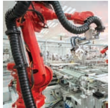
Modules are soldered either automatically by robots or manually by skilled employees on the same line.
