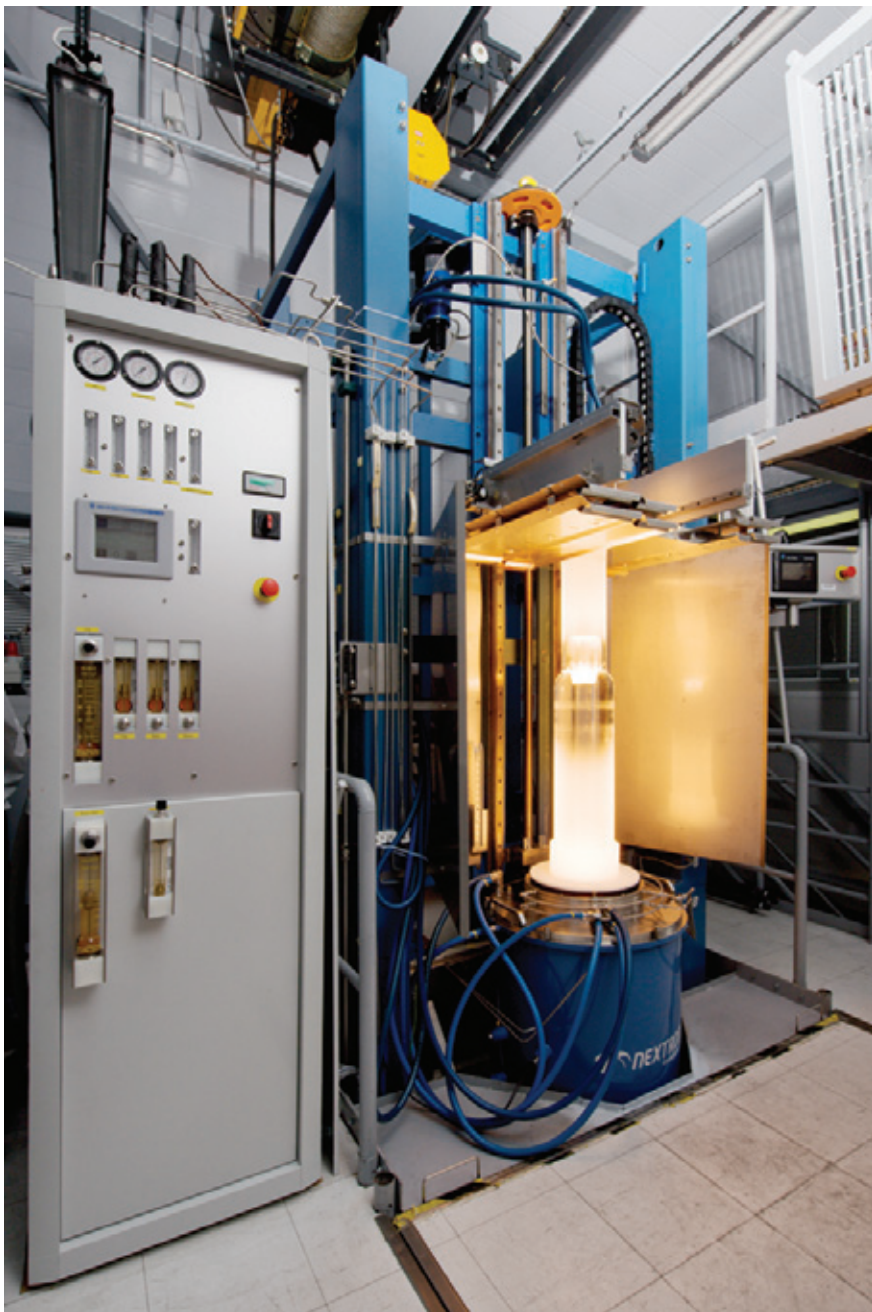
▲ The drawing of a 200mm diameter preform
