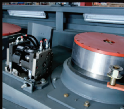
Multipass drawing line equipped with cassettes
