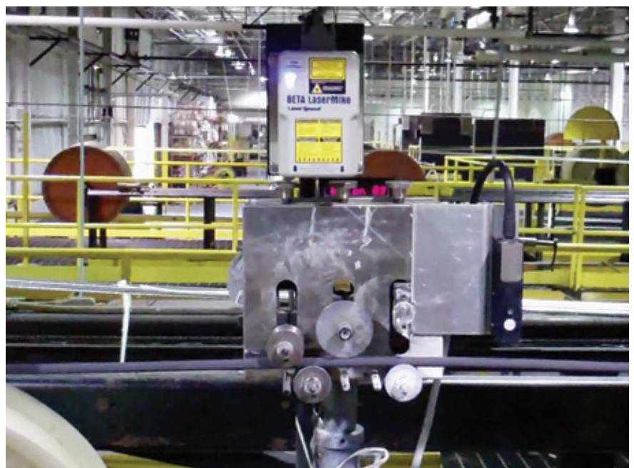
▲ LaserSpeed encoder alongside printing system before take-up reel
