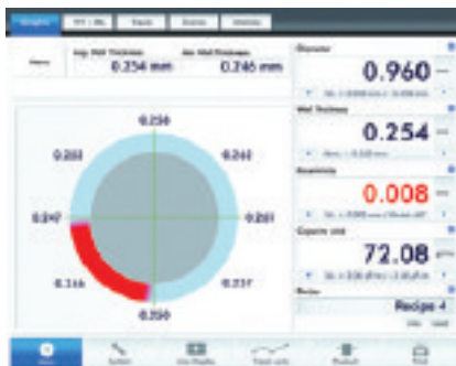
○ Standard representation of eccentricity at the Ecocontrol 2000
