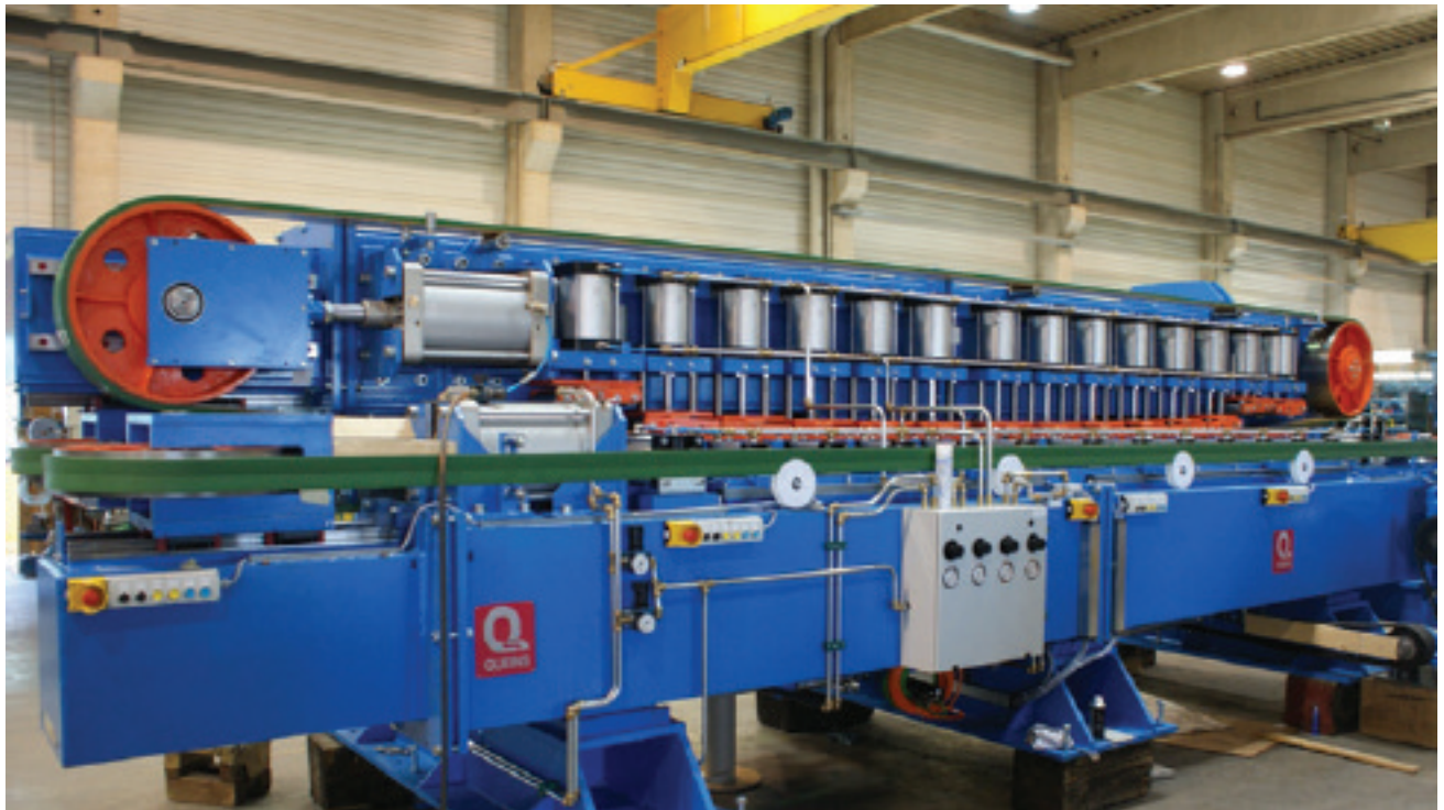
○ Above and below, the two heavy duty capstans supplied by Queins
