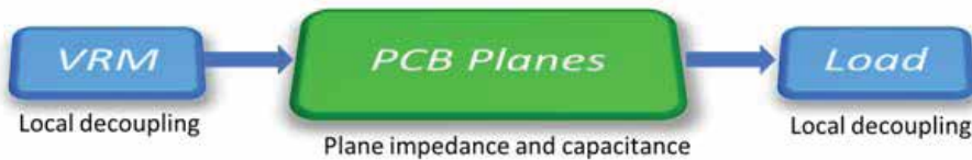
Figure 1. The Power Distribution Network (PDN) is comprised of the VRM, planes and decoupling capacitors
