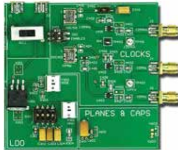
Figure 2. A section of the Picotest VRTS3 training board include an LDO (U301), bulk capacitors (C301-C304), a decoupling capacitor (C402) and a 125MHz clock (OSC401). The connections are made by PCB traces
