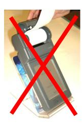
Paper incorrectly installed, remove till roll turn around and re-install!
