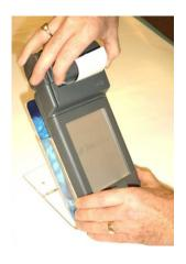
**1.** Grip either side of printer lid, squeeze and pull up.
