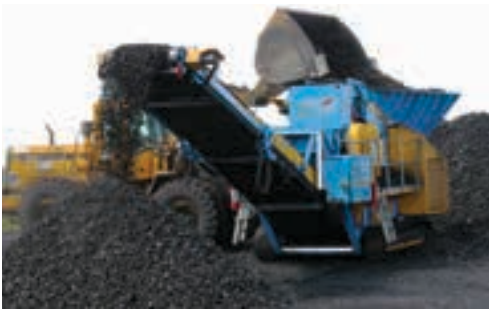
The DoppiaTrac is a track mounted, self-driven, feeding, crushing and stockpiling machine for medium to hard bituminous coal crushing applications.
