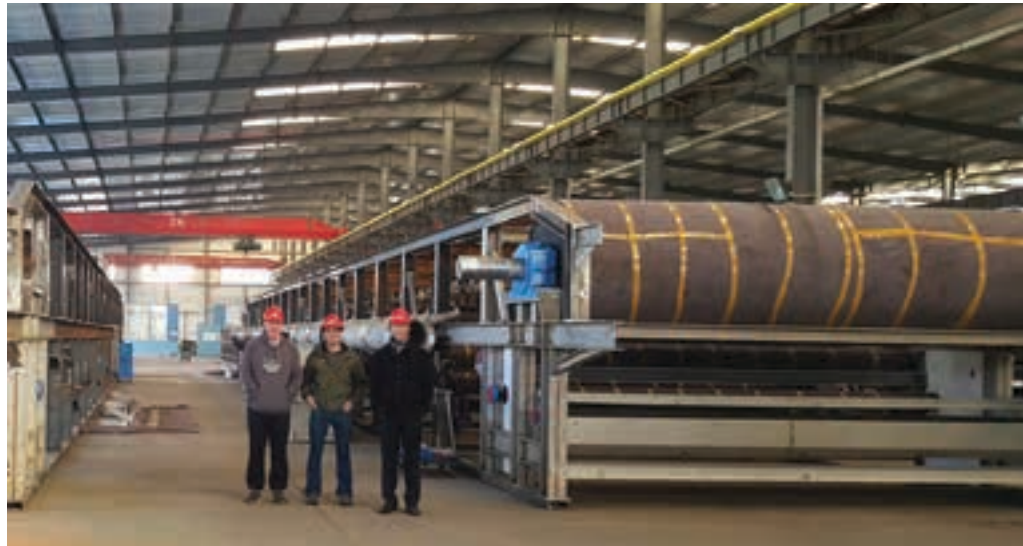
Shop assembly of 4 x 145 m 2 Roytec TXSY belt filters eight weeks after contract signature.
