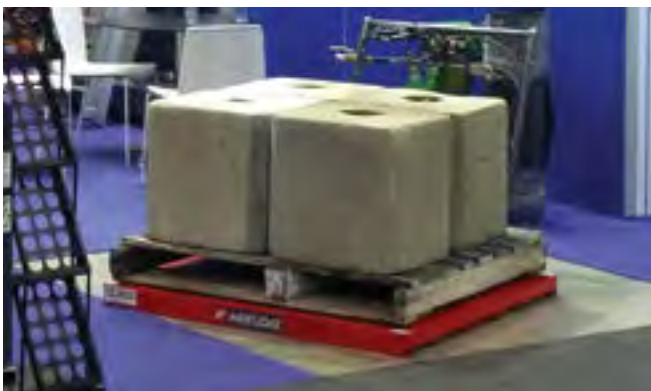
Pallet sized air skid with push handle
