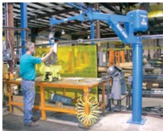
Easy Arm - an articulated jib crane with an in-built G-Force end effector.
