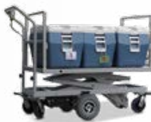
Customised version with power drive kit and railings fitted
