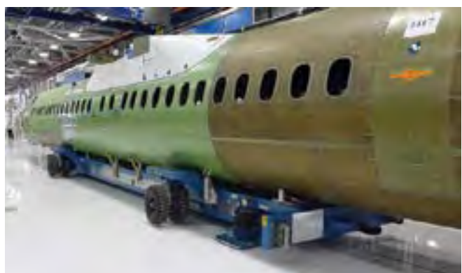
Air skids used to lift and move a dolly with product in a production line
