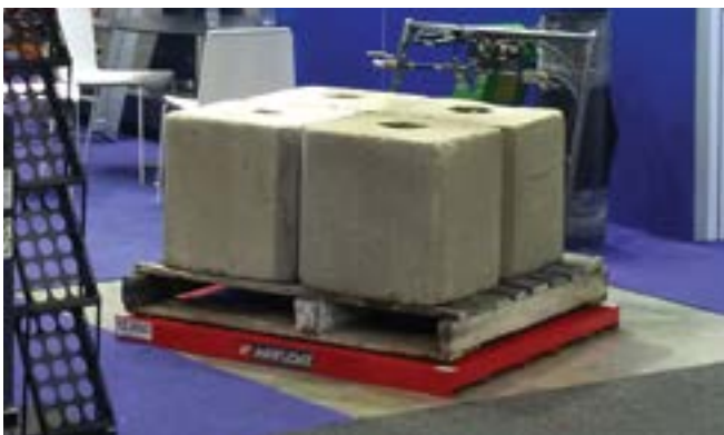
Pallet sized air skid with push handle
