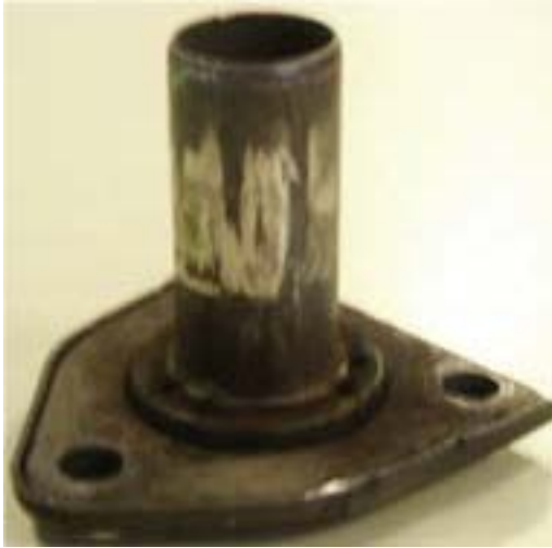
Typical worn guide tube – REPLACE
