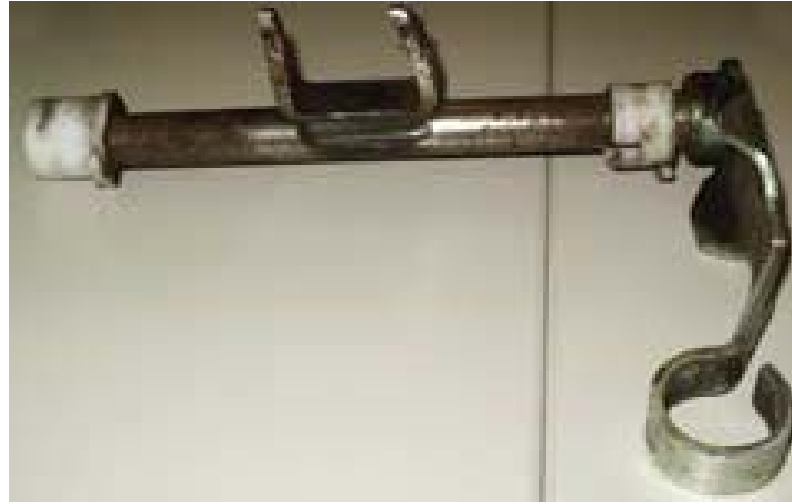
Cross shaft bushes worn – REPLACE
