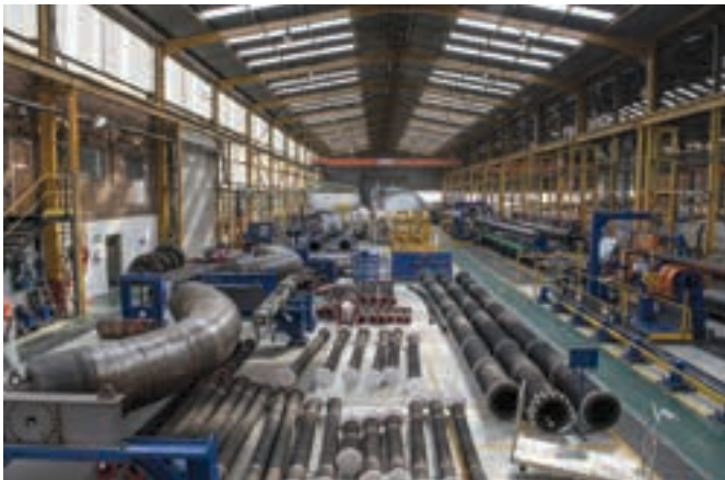
Left: Weir Minerals Africa's state-of-the-art hose manufacturing bay in Alrode, South Africa. Right: Weir Minerals Africa has installed six custom-built manufacturing lines for semi-automated hose manufacture.
