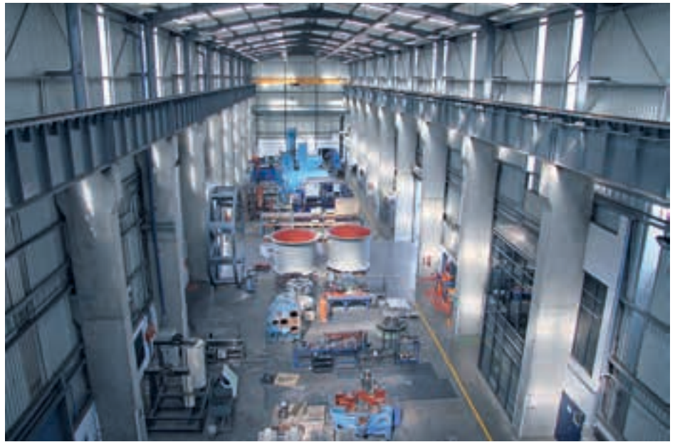
Above: The thyssenkrupp Industrial Solutions Service Centre in Chloorkop, originally equipped to manufacture and refurbish the largest Polysius-branded HPGRs, has CNC vertical and horizontal machining centres capable of handling 100 t components. Left: thyssenkrupp's coal-based circulating fluidised-bed combustion (CFBC) power stations operate at lower combustion temperatures and subcritical steam conditions. They can use much lower quality coal and discard coal, for example, which is normally regarded as unusable.
