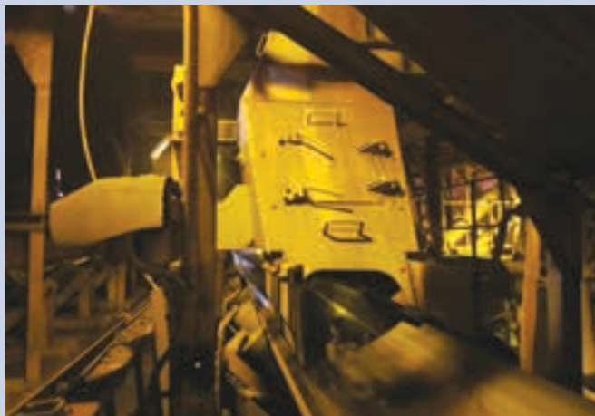
Above: Each Weba Chute System is custom designed to control the direction, flow and velocity of a calculated volume and type of material in each individual application.
