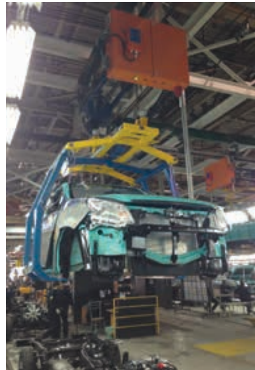
The assembly process saw automotive bodies and chassis from two separate production lines being joined on a single moving line.
