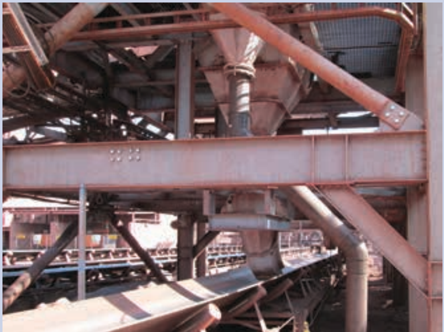
Above: Each Weba Chute System is custom designed to control the direction, flow and velocity of a calculated volume and type of material in each individual application.
