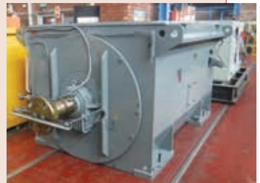
Marthinusen & Coutts recently completed the rebuild of a 6 550 kW, two-pole, 11 000 V squirrel cage induction blower motor for a copper mine in Zambia.
