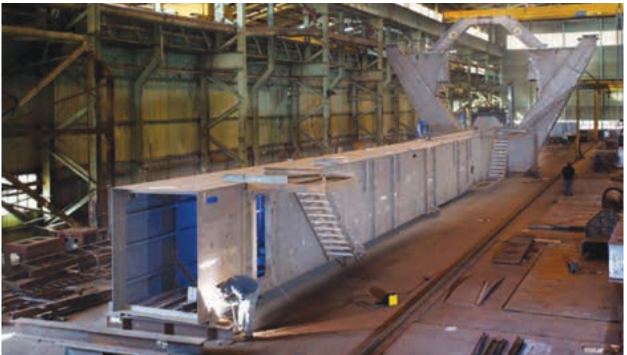
A ship loader crane leg being manufactured by DCD Heavy Engineering, which is part of the DCD Group's mining and energy cluster and is active in rail, defence and marine segments, offering comprehensive and integrated heavy engineering solutions.
