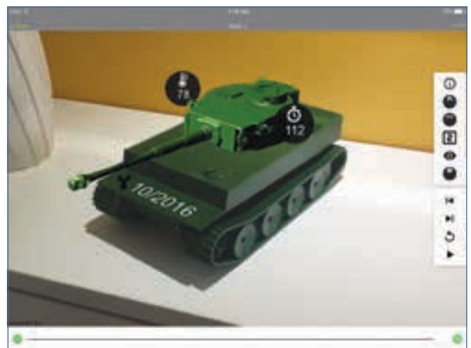
A 3D Vuforia model of the tank appears on the screen with a specific turret fitted, along with some background terrain. "We can now move around the terrain, mimicking the real tank's performance and we can change the turret to demonstrate to customer all of the different configurations incorporated into the design," Anderson tells MechTech .
