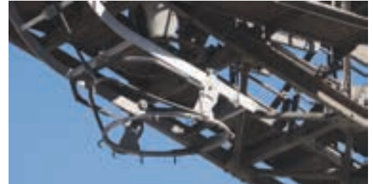
Introduced to address dust issues at conveyor discharge points, the R-SDR retractable stockpile dust ring was showcased as the latest innovation from I-CAT Dust Solutions.
