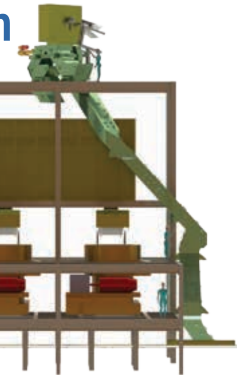
Among the challenges in this particular application was having to overcome a transfer height of 17.5 m by passing from just below the head pulley through the conveyor building, then under the structure, over the bin and down to the conveyor – and still provide access for crusher maintenance.
