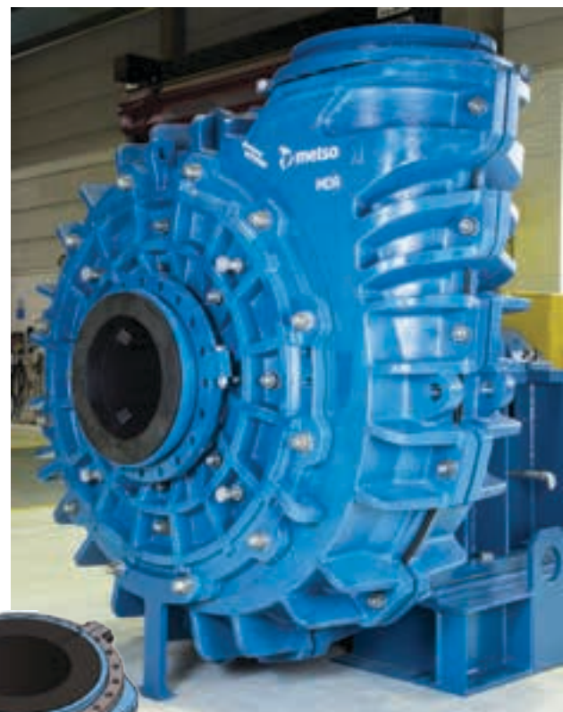
Above: The double adjust feature makes it easy to adjust the gap between the impeller and the inlet, making it easy to sustain the Metso MDR 300 pump's high efficiency.
