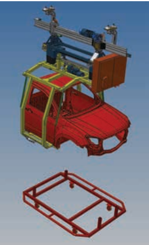
While a chassis is conveyed along the line, the Demag solution had to align a hoist above, fitted with a single cab and load box, travelling at a matching speed.
