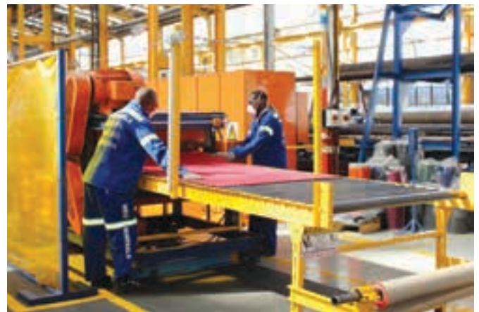
Left: To improve the accuracy, consistency and safety of liner cutting, Weir Minerals uses a CNC AquaCut water jet cutting system to cut Linatex sheet into the rubber shapes required. Right: Linatex premium rubber sheeting is passed through a buffing machine to roughen the surfaces.
