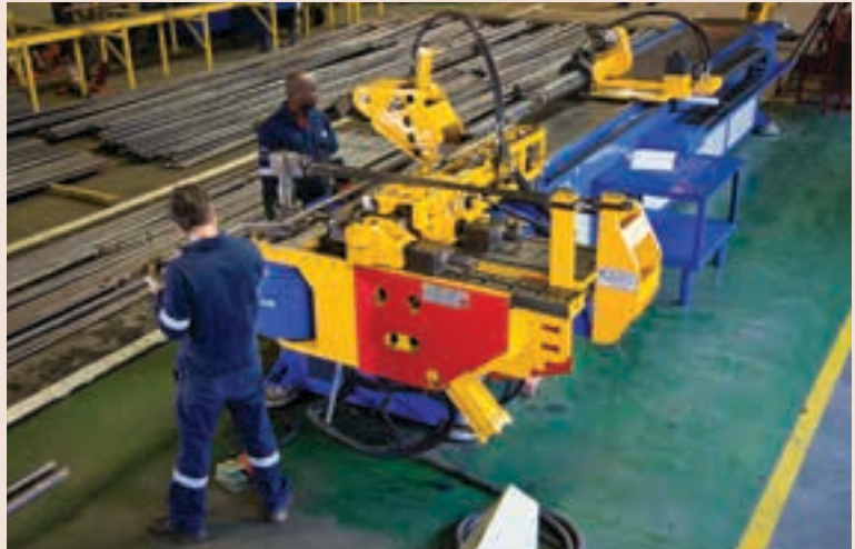
Babcock recently invested in a new, fully automatic, CNC bending machine for manufacturing steam generation parts as part of a drive to improve efficiencies at its Jet Park, Boksburg fabrication facility.
