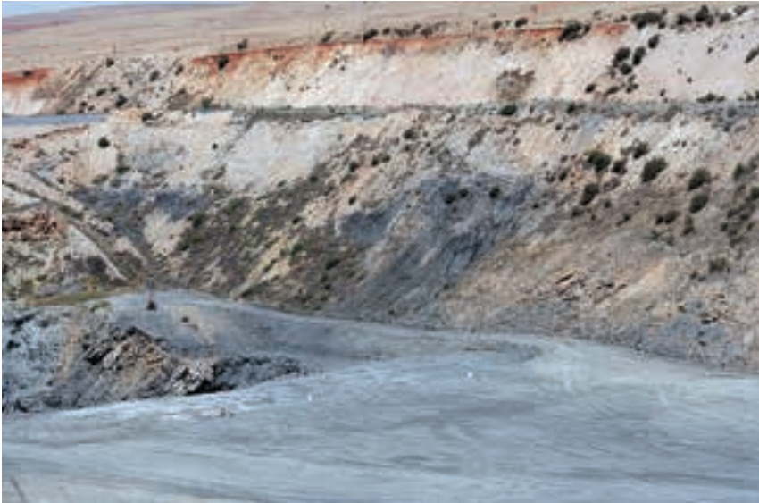
The new Vondeling pit, which commenced mining in 2007, is at a current depth of 50 m. One can see the sump established at the back, and the next cut will be into the limestone. In the short to medium term, the plan is to extend the front area because of the shallow limestone deposit. In the front one can see the overburden and a small amount of limestone in the corners, with the majority of the limestone being on the lower level.
