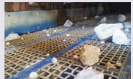
Woven wire polyurethane surround panels from FLSmidth, which has been operating successfully in Africa for over a century.
