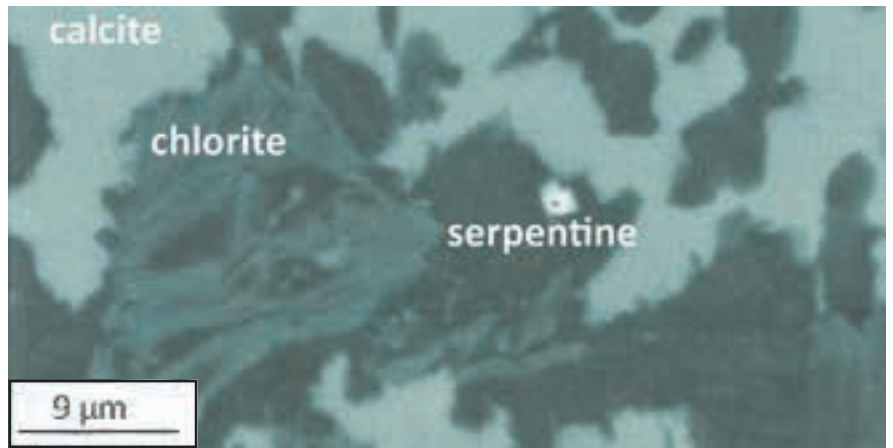
Figure 3: Illustrates a backscattered electron image showing the distribution of calcite, serpentine and chlorite.
