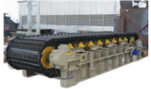
The apron feeder for Petra Diamonds' Williamson mine in Tanzania.
