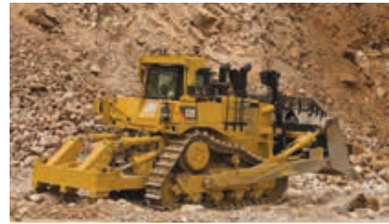
Engineered for maximum production and service life: the Cat D10T2's mainframes are built to absorb high impact shock loads and twisting forces encountered during severe dozing and ripping applications.
