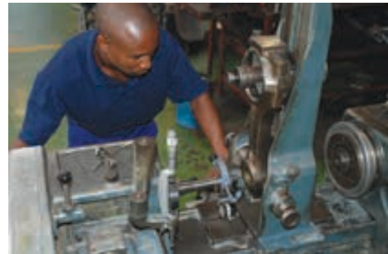
Small-end bush machining at Metric Automotive Engineering's facility.
