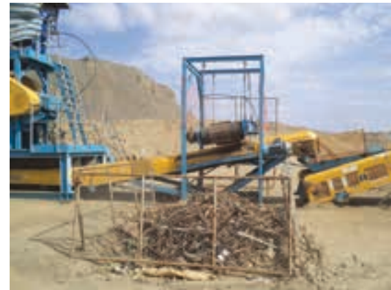
Above: The addition of an overband magnet to a modular plant or conveyor system is a customer's insurance policy against the risks of mechanical damage and downtime.
