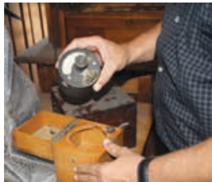
A pyrometer, still in its beautiful hand-made wooden box, which is stored in a leather case.
