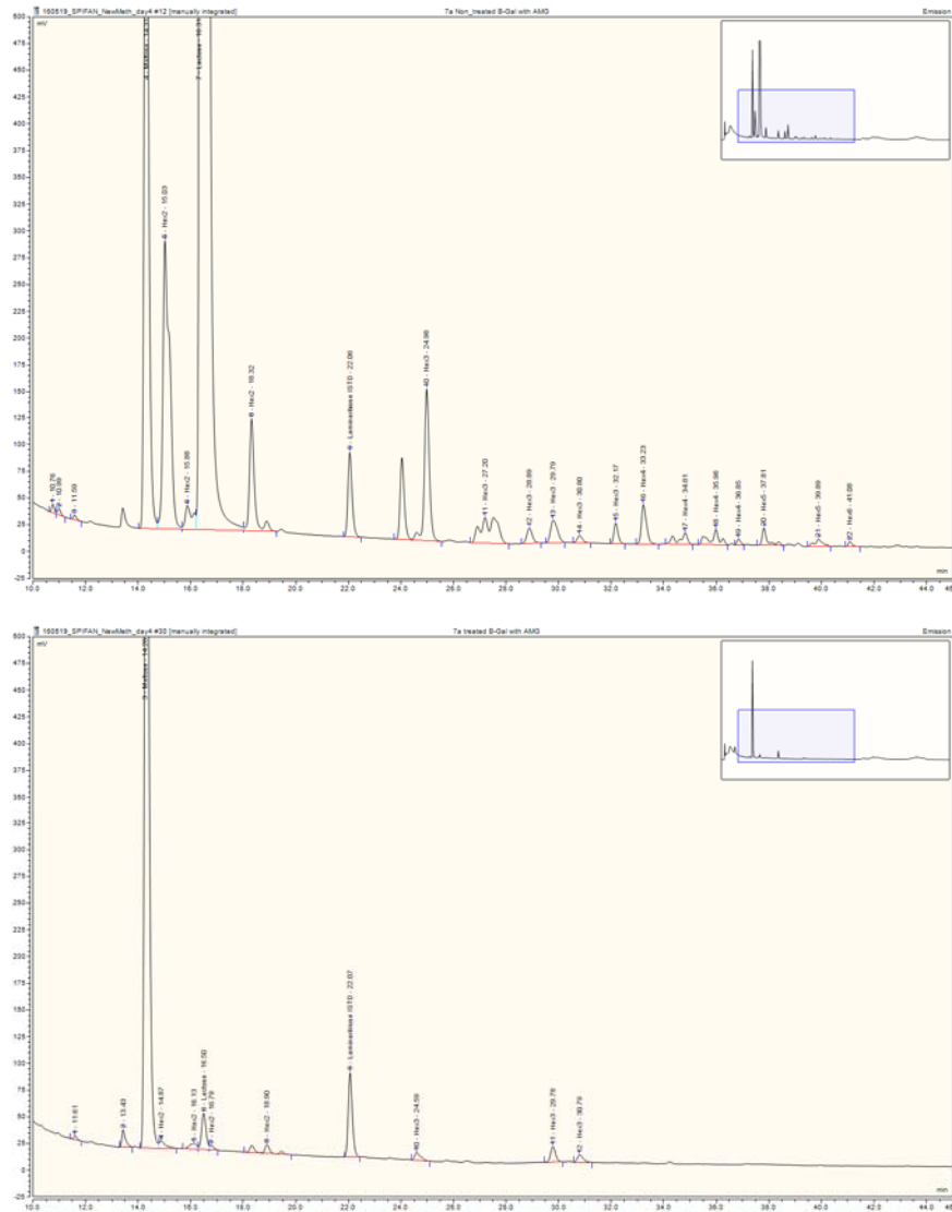
Figure 5: Chromatograms of Infant Formula Powder Partially Hydrolysed Milk Based Containing 0.33 g/100g GOS. Upper Chromatogram Untreated, Lower Chromatogram After \beta -Galactosidase Treatment.
