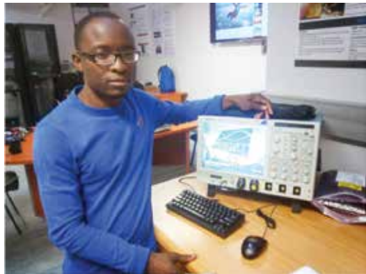
Dr. Chamunorwa Oscar Kureba, Postdoctoral Research Fellow, WITS HEP Group, with the Tektronix MSO70804C – 8 GHz 25GSa/s Mixed Signal Oscilloscope shortly after successful installation.
