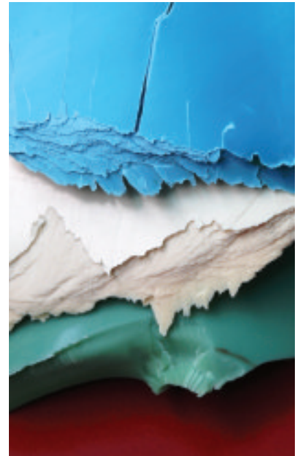
Amorphous PVC-U structure (green in colour), subjected to molecular orientation adopts a layered structure. The higher the orientation class, the more defined layers there will be (blue section class 500, and white section class 400)
