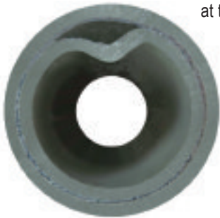
The X-Ray 6000 Triax detects defects between the vapour barrier and the inner tube
