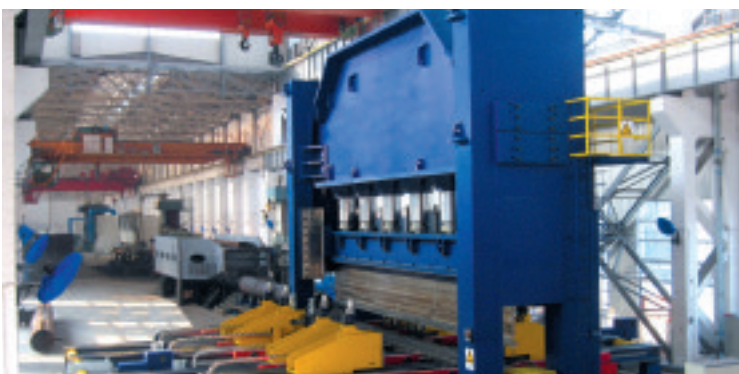
52,000KN JCO Forming Press
