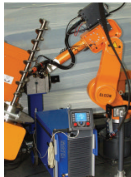
ⓘ Qineo Pulse pulsed arc power source with portable remote control for flexible use with Romat® industrial robots
