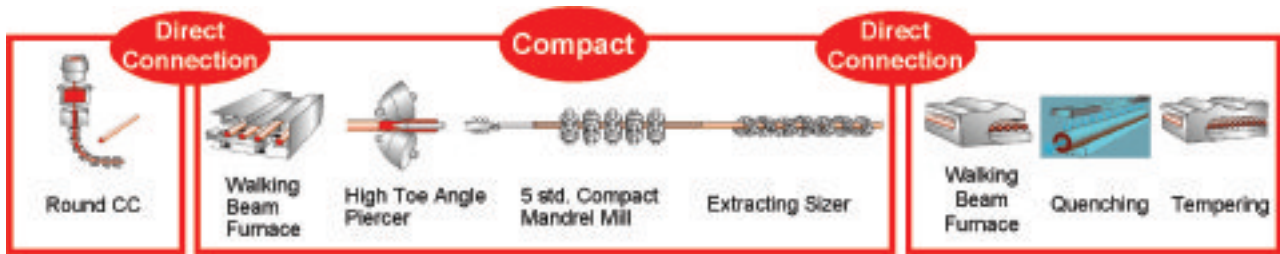
Figure 1-b: Schematic illustration of the simple and compact medium size mill and inline heat treatment facilities
