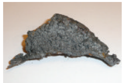
Cutting burr removed from the billet
