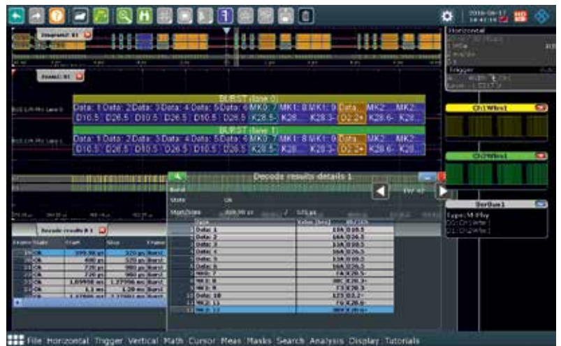
Fig. 10: M-PHY layer decoding results with zoom and table display the details of the frames and bursts (source: Rohde & Schwarz).
