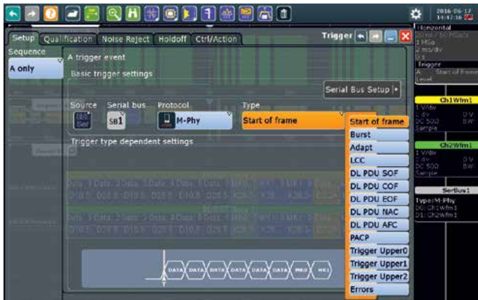
Fig. 11: M-PHY / UniPro protocol decoding setup (source: Rohde & Schwarz).
