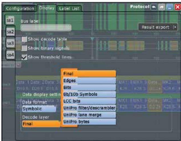
Fig. 9: Selection of the decoded layer (source: Rohde & Schwarz).
