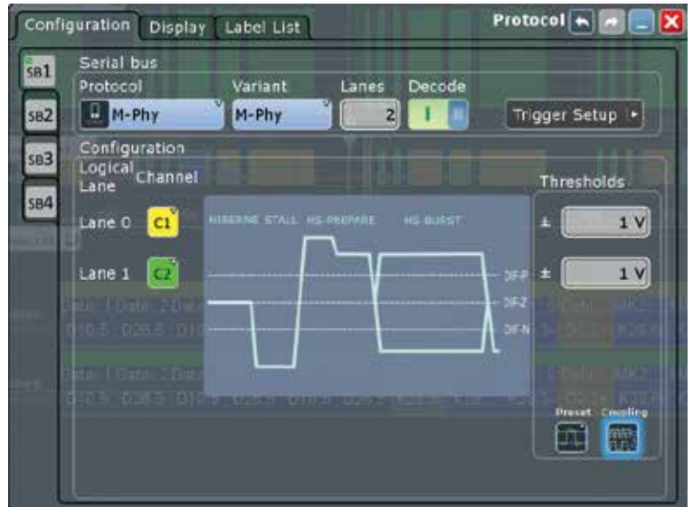
Fig. 8: Configuration of M-PHY / UniPro protocol decoding (source: Rohde & Schwarz).
