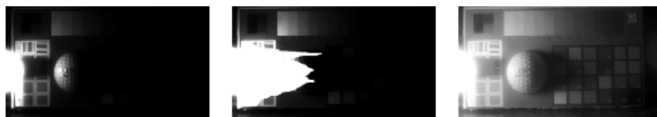
Figure 2: A scene with both bright and very dark components, imaged by a standard IT-CCD (left), a standard EMCCD (center), and an Interline Transfer EMCCD device (right)
