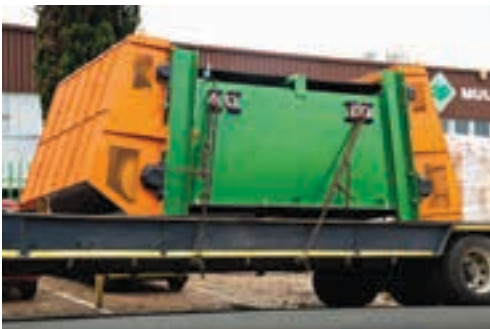
Longi-Multotec's standard range of air-cooled magnets goes up to a 30-t machine.
