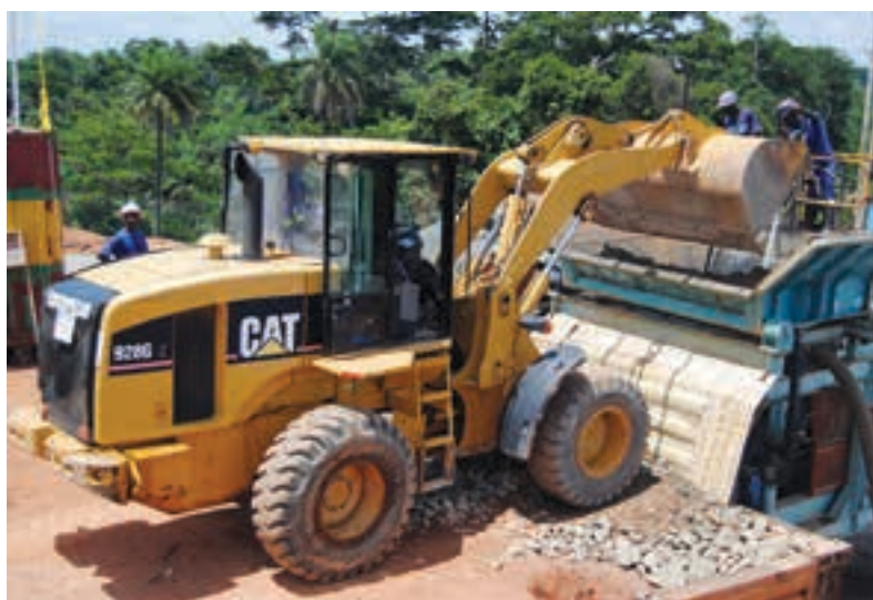
Loading ore into the Tongo plant as part of bulk sampling operations.
