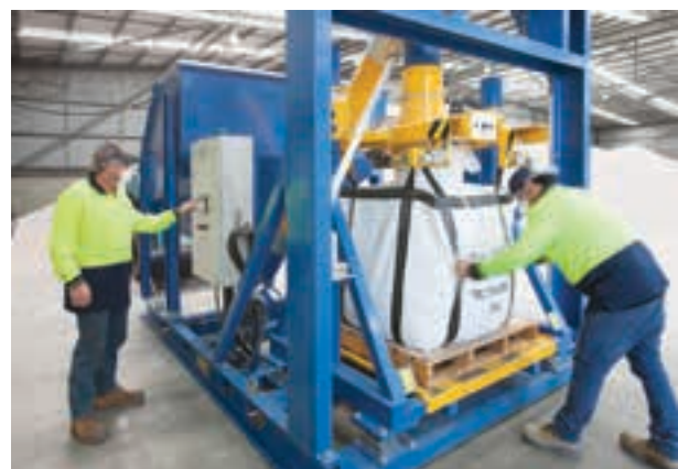
One operator attaches the bag to the fill head as the other operator pre-sets the bag weight and initiates filling at the PLC. The Twin-Centrepost™ design filler frame and heavy-duty outer frame impart strength for filling bags weighing between 1 000 and 2 000 kg.
