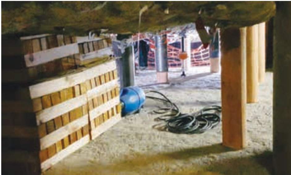
Measuring some 7 m long, the model stope dips at 10 degrees, has a stoping width of 1 m and extends some 3 m on strike. It has been equipped with various items of support infrastructure to demonstrate to students the variety of technologies employed underground (photo: Arthur Tassell).
