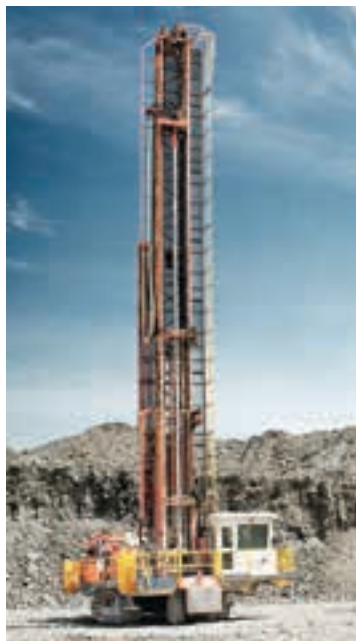
The Sandvik DR461i blasthole drill rig.
