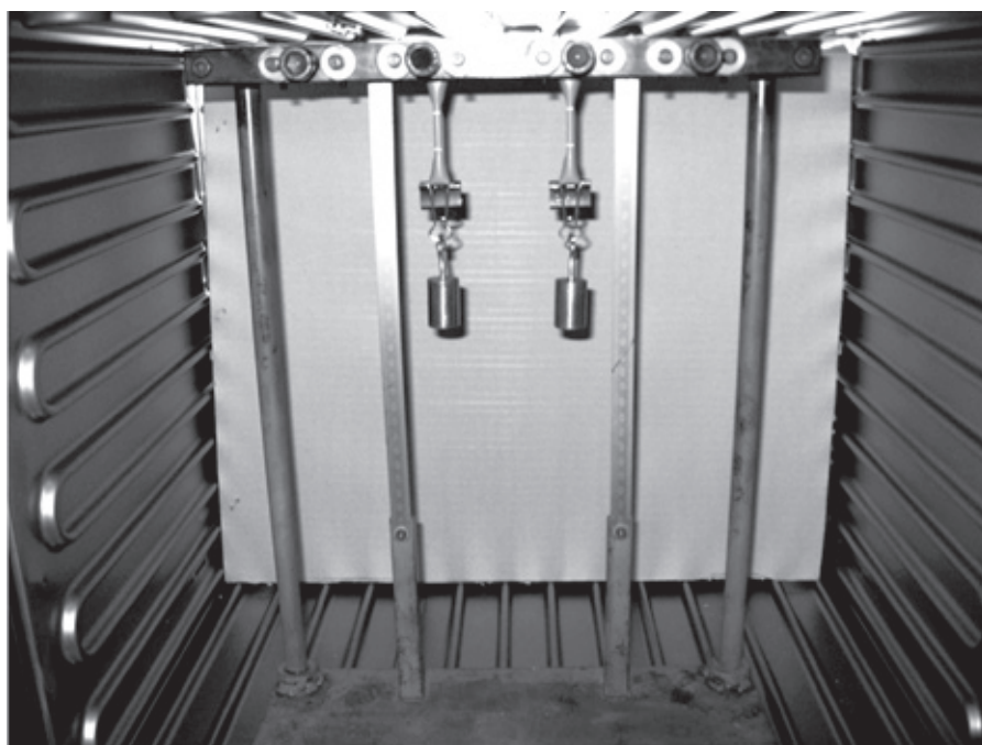
○ Figure 2: Hot elongation test
