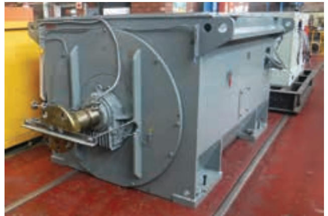
Marthinusen & Coutts recently completed the rebuild of a 6 550 kW, two-pole 11 000 volt squirrel cage induction blower motor for a copper mine in Zambia.
