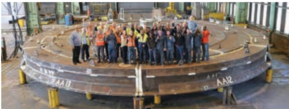
The 380-ton base for the dragline excavator.
