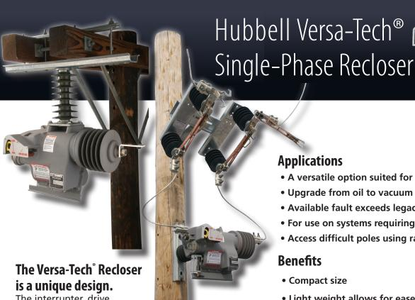
The interrupter, drive mechanism, control, and housing are raised to the system potential. The entire assembly is then insulated from ground using a standard polymer post insulator. This compact simplified design eliminates the potential for an insulation breakdown failure.
