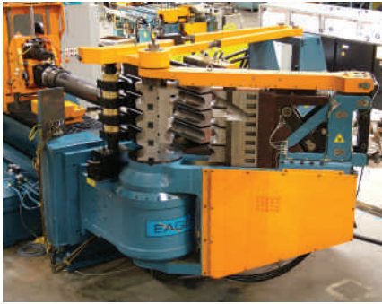
ⓘ The bender is designed to handle heavy wall schedule 80 pipes of 30ft in length and up to Ø 3.5"
