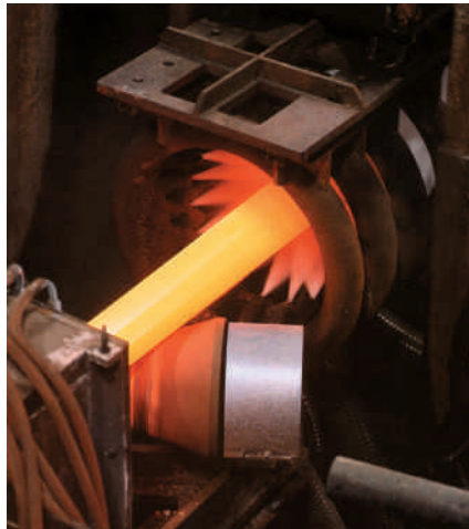
Ⓜ Heating a pipe using machinery from Ajax Tocco
