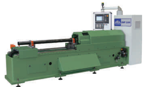
ⓘ Arla end-working machine for pipe, tube and shaft
