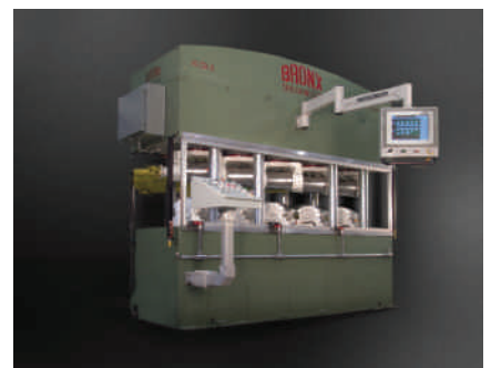
Ⓢ Bronx/Taylor-Wilson's tube straightening machine is available in 6 and 10 roll configurations
