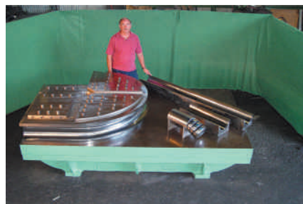
Eaton Leonard Tooling manufactures large diameter bender tooling
