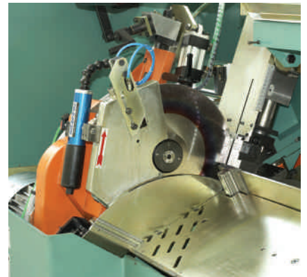
Ⓜ The cutting head of the MCL 120 IMS
