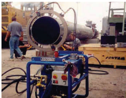
Protém's portable tube cutting and pipe bevelling machine
