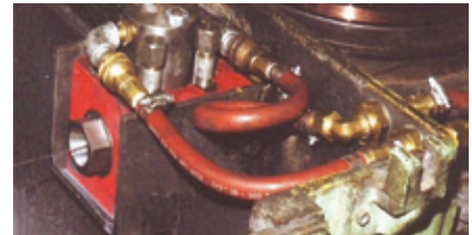
▲ Wire cleaning by PWC-S system
