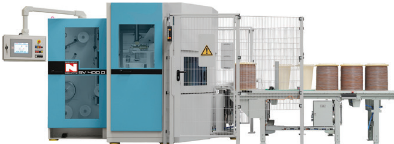
▲ SV 400 D type double spooler for insulated wires with filled and empty spools (Niehoff Package System)
