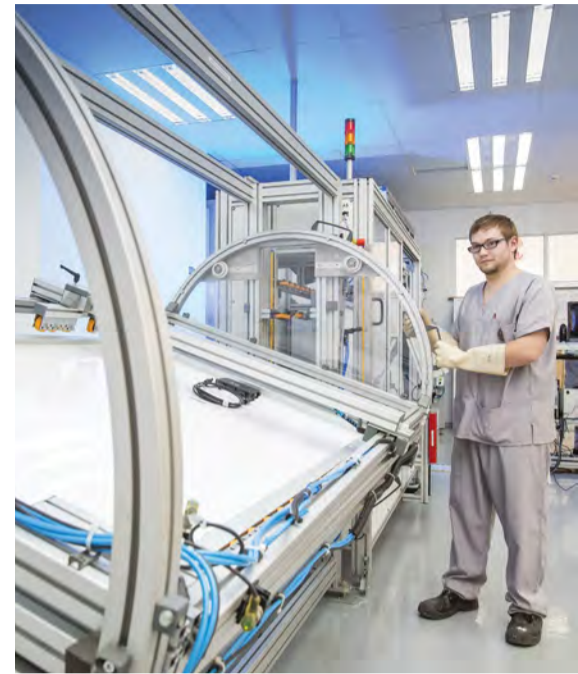
These PV modules were manufactured at the ARTsolar plant in New Germany, KwaZulu-Natal, for the Mulilo Sonnedix Prieska PV solar plant project. Liam McIntosh is responsible here for framed PV modules, which are rotated into a vertical orientation for earth leakage and sun simulation testing.
