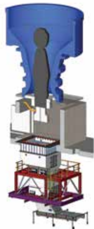
An illustration of the Weba Chute System custom engineered transfer point at a diamond mine.
