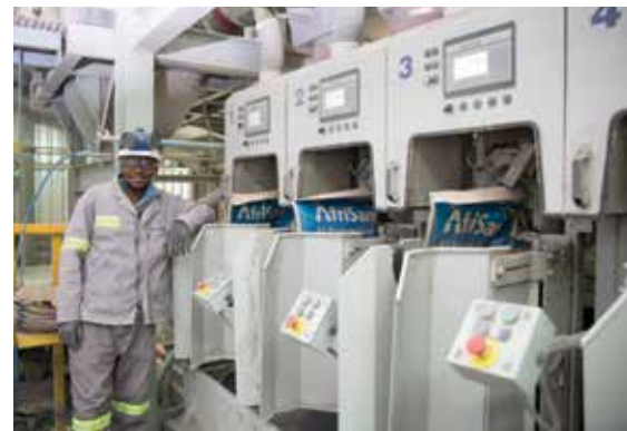
The packer – a 60 t/ hour, four spout in-line European design – is utilised in series with a robotic arm palletiser to pack and stack the cement bags.
