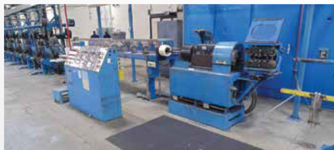
Tensor SZ Cabling Line
