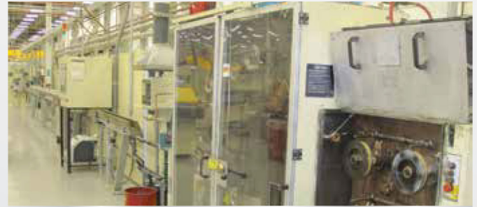
60mm Nokia/Niehoff Tandem Wire Insulating Line
