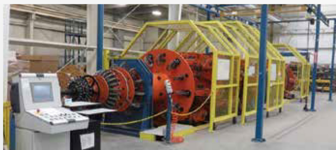
630mm Cortinovis Planetary Line 6+18
