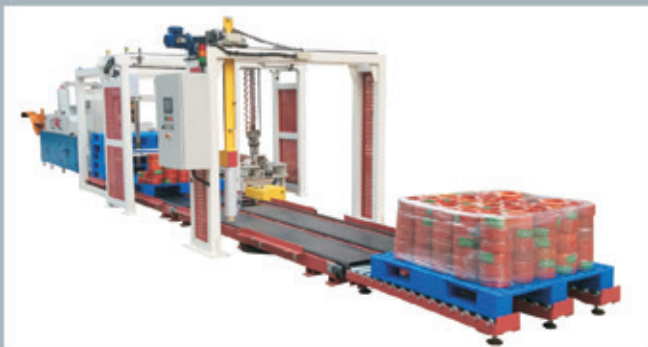
Auto coiling and stacking line
