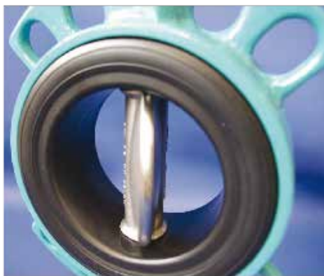
BFV DN 80 after running 20 000 opening/closing cycles
