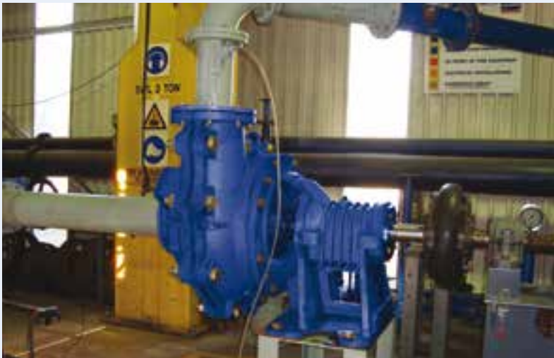
The Warman WBH slurry pump undergoing testing at the Alrode manufacturing centre.
