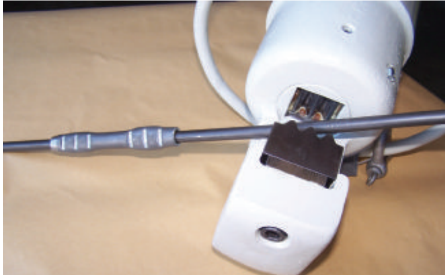
▲ Petig's Hydrocut used to join wire ends by crimping
