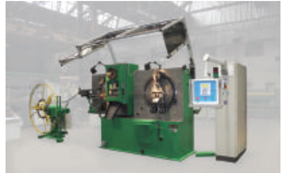
▲ Bend-50 CNC – automatic wire and strip forming machine
