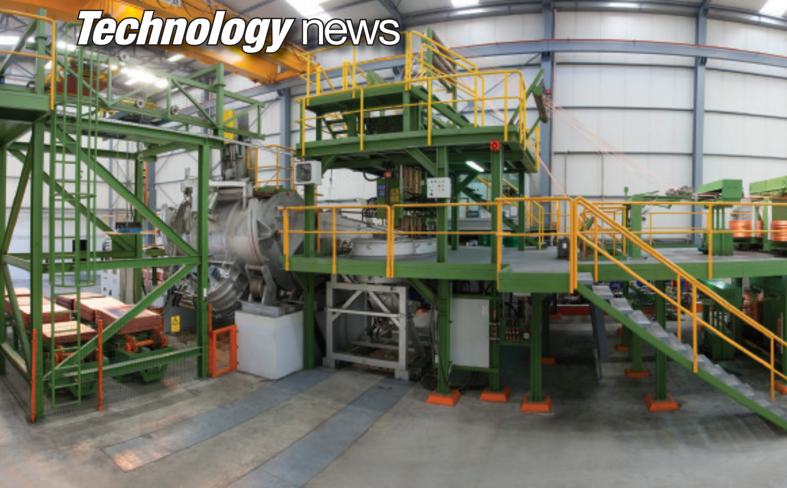
○ The double-furnace casting line supplied to Vatan Kablo, Turkey
