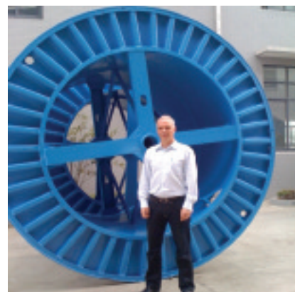
○ Inosym's largest reels are designed to carry 25,000kg
