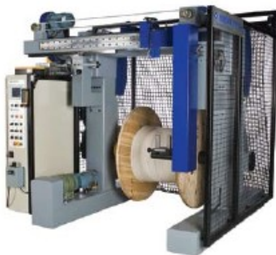
○ Take-up UW16HD with integrated laying unit, remote control and safety guarding
