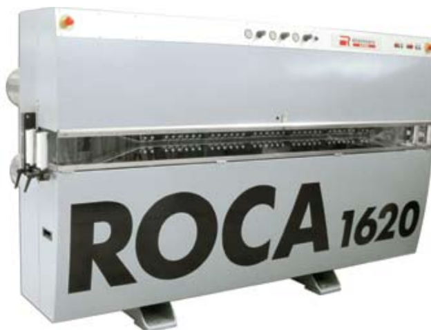
○ The new ROCA caterpillar for medium and large cables
