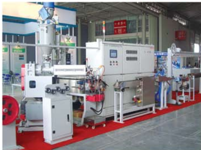
70+60 高精度双层共挤挤出机生产线 70+60 Double layers co-extrude extruder line
