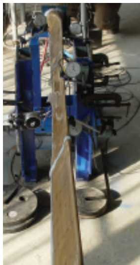
Figure 18: Three wave mode of specimen A0 in experimental study
