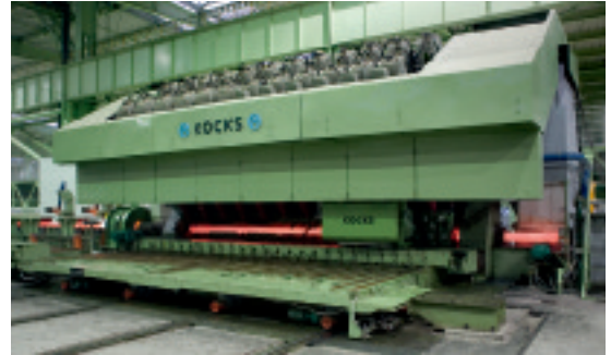
The machinery produces tubes up to a diameter of 177.7mm
