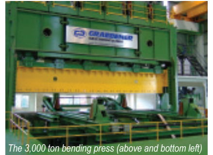
The 3,000 ton bending press (above and bottom left)
