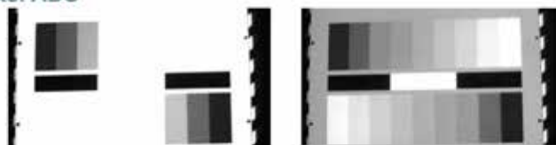
Figure 7: Piece-wise linear forming of the sensor response curve achieves a higher dynamic range
