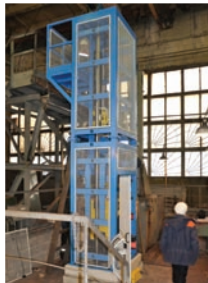
Imatek has installed a DWT40-30 drop weight tear tester at Ural Steel
