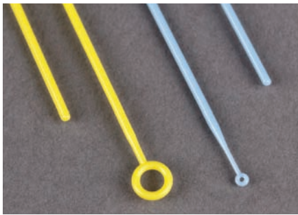
Loops feature integrated needle at reverse end
