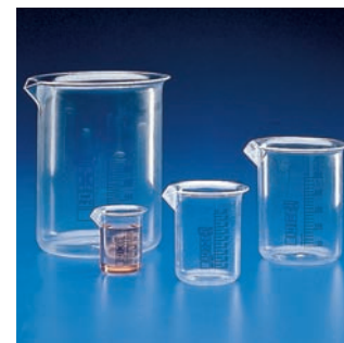
Polymethylpentene (PMP) with Printed Graduations
