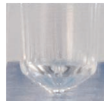
Conical Bottom (V) Each well is 250 \mu L
