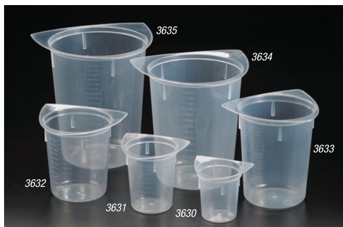
Clarified polypropylene tri-corner beakers
