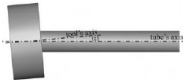
Figure 7: Tool position regarding to the tube's axis
