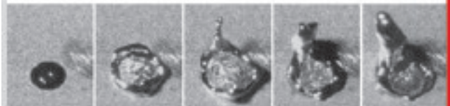
Nd:YAG laser welding - Development of the keyhole. Image series taken with frame rate of over 1000 frames/s.
