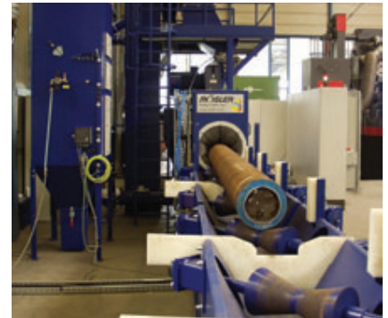
Tubes are transferred into the shot blast machine
