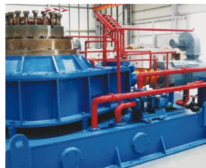
▼ Sinoleader's continuous lead sheathing extruder
