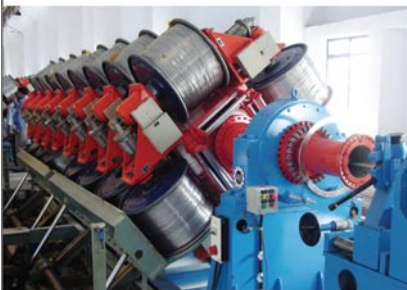
Rigid Wire Stranding Machine with Auto Batch Loading System
