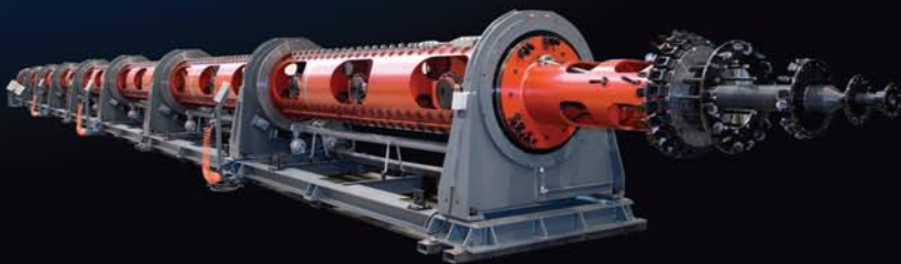
Tubular strander for copper, aluminium or steel wires
