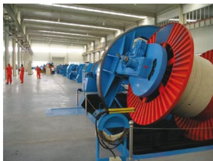
▲ Pourtier Drum Twister line for power cable DTPC 1600... 5000
