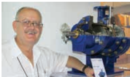
Jan van Vuuren of KSB Pumps and Valves with a cut-away RPHmdp mag drive pump for use in hazardous applications.
