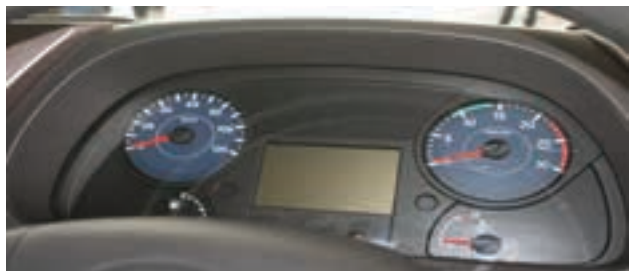
Above: The ergonomic layout of the dashboard increases the safety on the road. The large 4.5-inch display ensures readability and displays information on UD's innovative fuel coaching system. Left: The range for southern Africa includes 13 model derivatives, including freight carriers, truck tractors, rigids and specific construction applications such as tippers, tankers and mixers.
