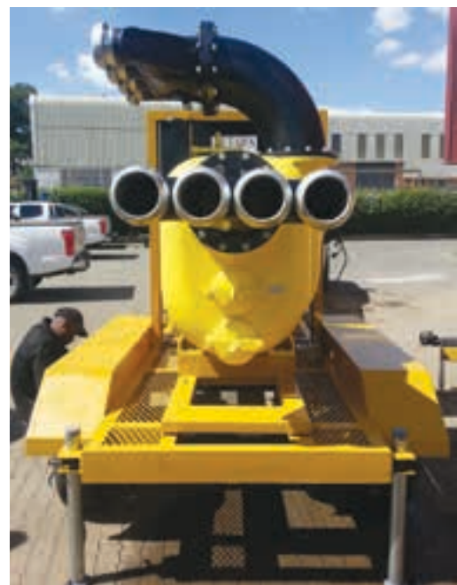
Letaba Dewatering also builds trailer pumps, the largest being the Zambezi unit, which has a diesel driven Varisco J 12-400 dewatering pump.
