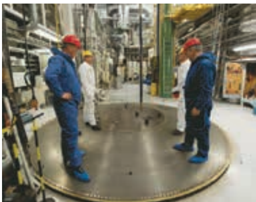
Norway-based Thor Energy's test rig containing six thorium fuel rods being installed in the IFE Halden Research Reactor. Photo: T.Tandberg
