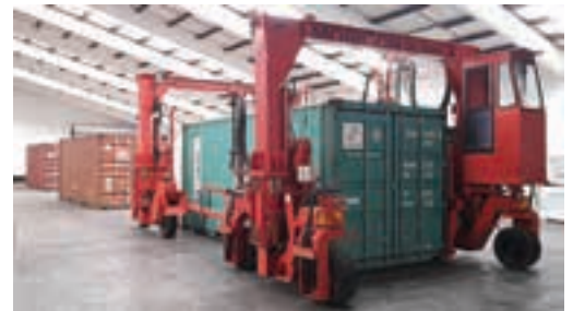
The Mobicon mobile container handler, with a 33 T lift capacity, has increased operational efficiency at the plant and reduced demurrage costs for trucks waiting to be loaded and unloaded.
