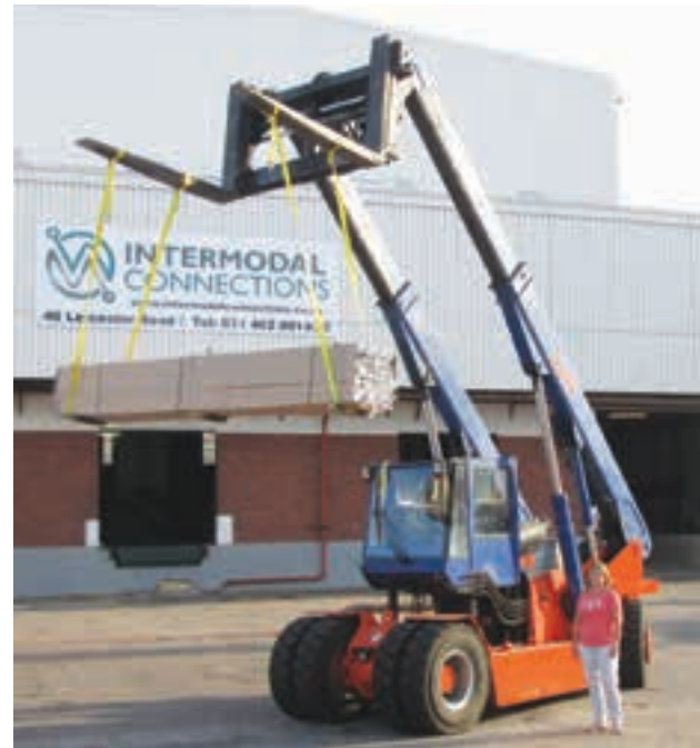
Jo-Ann Mellon, Intermodal Connections' managing director, with a Meclift variable reach truck offloading 26 bundles of aluminium profiles.
