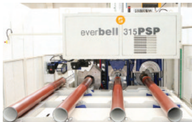
▲ Sica's Everbell/H 315 PSP automatic belling machine
