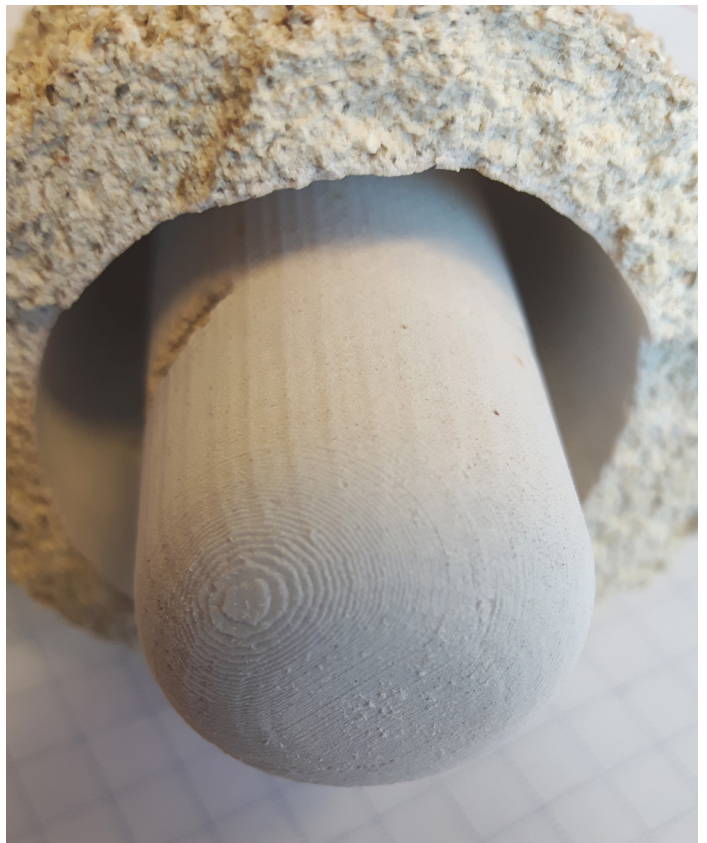
Checking the burnout of PLA/PHA Natural, breaking the mold to inspect pattern for residue. Patterns printed on the Stacker S4, 0.2mm layerheight at 20% infill.
