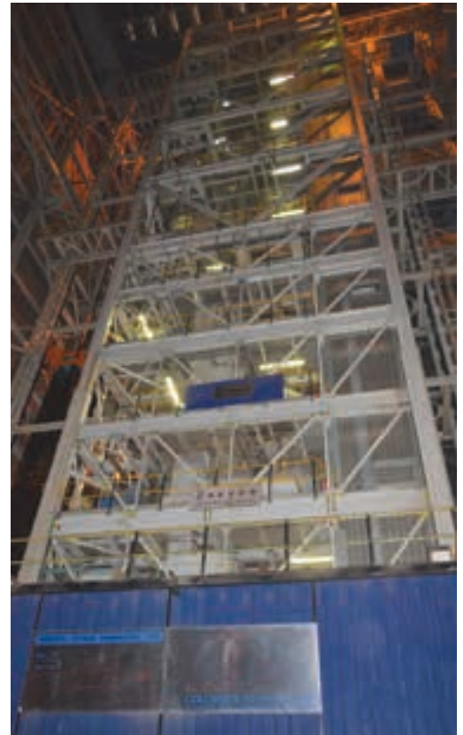
The VBA vertical furnace where a bright annealed (BA) finish is produced.
