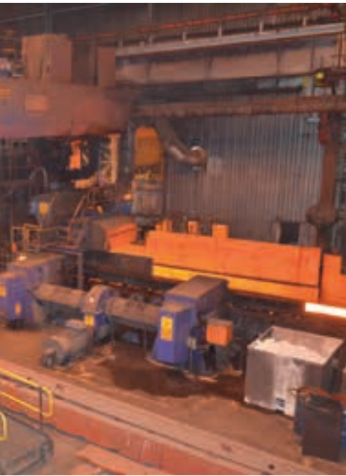
Left: Following reheating to between 1 100 and 1 300°C, depending on the stainless steel grade, the slabs are rolled on a reversing four-high mill to gauges of between 65 and 25 mm. Above: Cold rolling of the No. 1 coils takes place on one of four Sendzimer mills (Z-mills), which produce smooth, shiny finished, cold rolled stainless steel. The thickness range of the cold rolled product is between 0.2 mm and 6.0 mm. Below: The rolled material is then annealed (softened), pickled and passivated, before it is processed through the skinpass mill, to ensure a smooth surface, known as a 2B finish.
