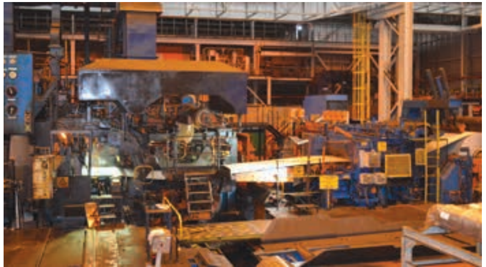
Left: Following reheating to between 1 100 and 1 300°C, depending on the stainless steel grade, the slabs are rolled on a reversing four-high mill to gauges of between 65 and 25 mm. Above: Cold rolling of the No. 1 coils takes place on one of four Sendzimer mills (Z-mills), which produce smooth, shiny finished, cold rolled stainless steel. The thickness range of the cold rolled product is between 0.2 mm and 6.0 mm. Below: The rolled material is then annealed (softened), pickled and passivated, before it is processed through the skinpass mill, to ensure a smooth surface, known as a 2B finish.
