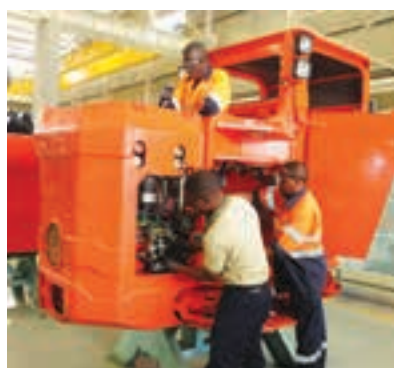
Technicians rebuilding an LH514 underground loader at Sandvik's new support centre in Zambia.
