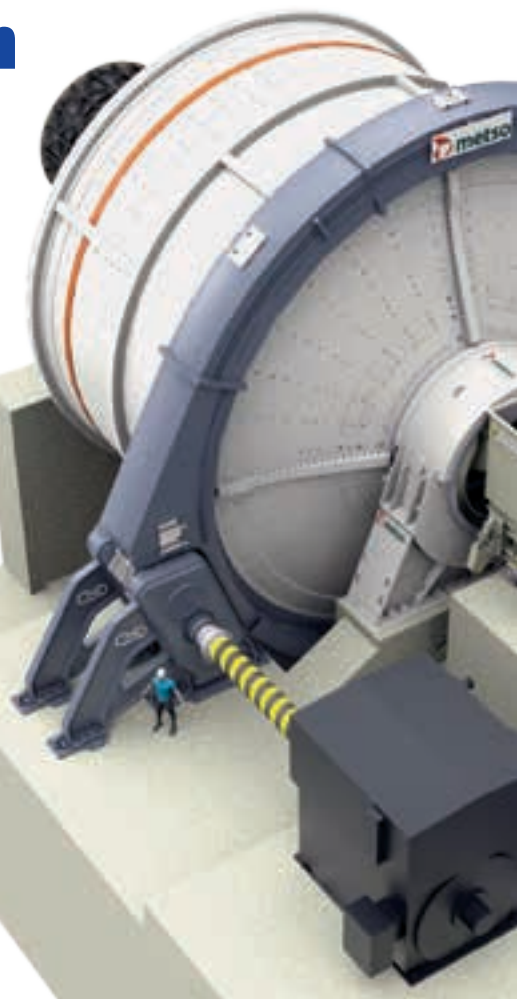
Metso's QdX4 Mill Drive system rearranges the dual pinion arrangement into a quad system that equally divides input power from two load-sharing motors into four pinions.
