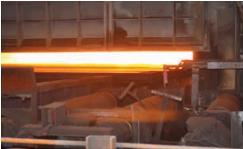
A slab in the re-heat furnace being prepared for hot rolling.
