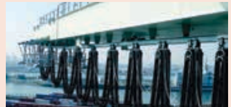
Cable festoon systems from Powermite are critical for materials handling machines that require efficient distribution of power, data, air or fluids.
