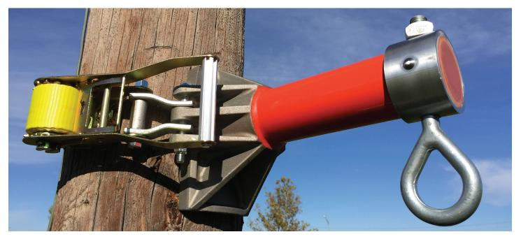
Provides insulation/Isolation from differences in potential by means of the 6" Epoxiglas link Meets 5,000 lb. requirement as specified by OSHA 1910.66 App C personal fall arrest requirements
