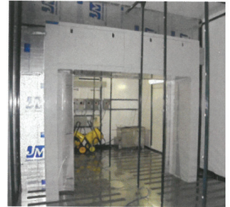
The HCR calorimetric environmental test chamber at CTS Labs in Urbana, IL
