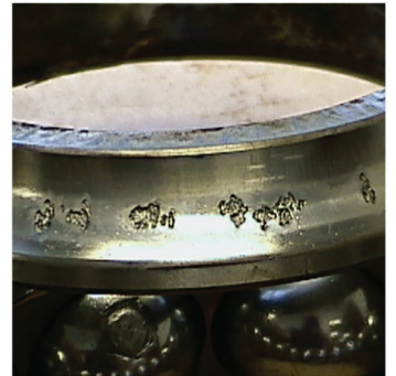
Unusual failure mode caused by breakdown of oil additive after only 9 months in operation.
