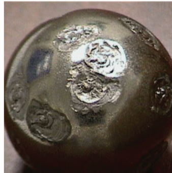
Unusual failure mode caused by breakdown of oil additive after only 9 months in operation.
