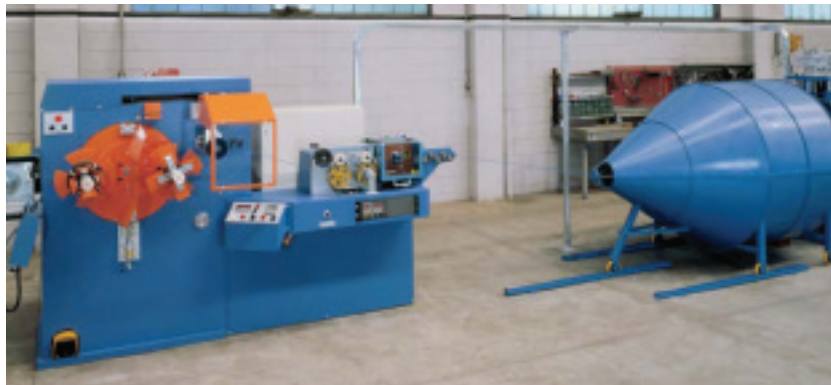
○ PS 80 semi-automatic coiling line
