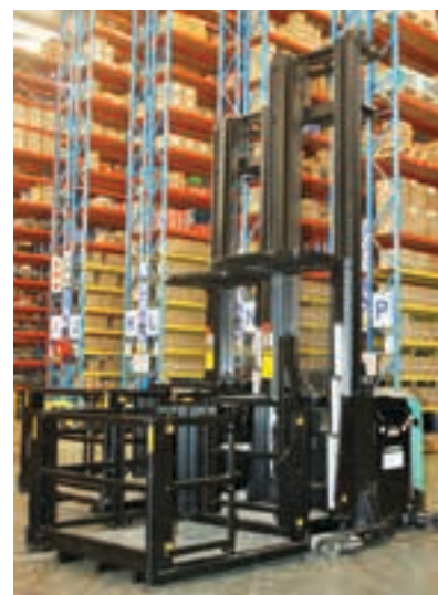
Bearings International's new forklifts have a higher load capacity of 2.0 t and a reach of 13 m.
