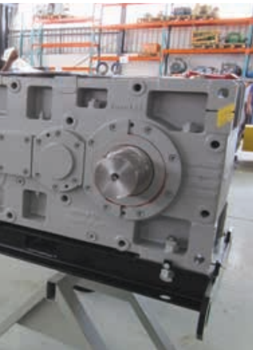
Above: A Bonfiglioli 300-series planetary drive under test at Bonfiglioli’s ISO 9001: 2008 accredited Linbro Park assembly facility.
