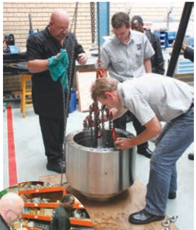
BMG's expanded facility includes specialist assembly and repair workshops for drives, conveyors, hydraulics and pneumatics, as well as electric motors, electronics, gaskets, lubrication systems and filtration. Left: Application of lubrication on a Tsubaki backstop. Above: A Tsubaki backstop component is being assembled.
