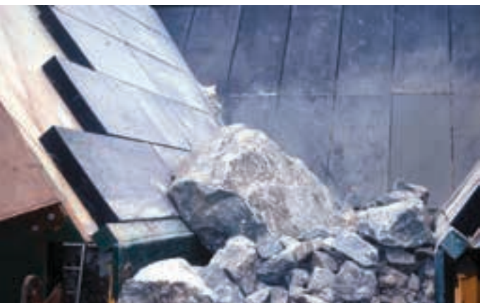
Truck bed linings are used in the haul truck box to protect it and the entire truck structure from wear and damage while transporting rock from the mining pit.
