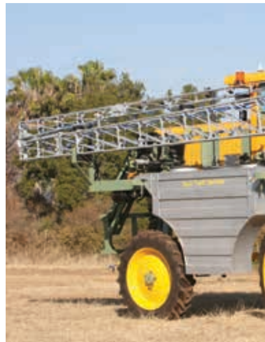
A Peake Mk3a dual-tank crop sprayer manufactured by Peake Equipment near Brits in South Africa. As well as incorporating hydrostatic steering for two- and four-wheeled steering, these machines use Black Bruin hydraulic wheel motors to deliver torque to all four wheels. A diesel engine drives the SAM Hydraulik pump to power the hydraulic circuits and SUN Hydraulics cartridge valves in a manifold block supplied by Axiom Hydraulics are used for control.
