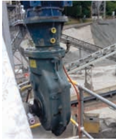
Dodge motorised torque arm units (MTAs) are used in industries where a shaft-mounted reducer is required particularly in the quarrying and aggregate sectors.
