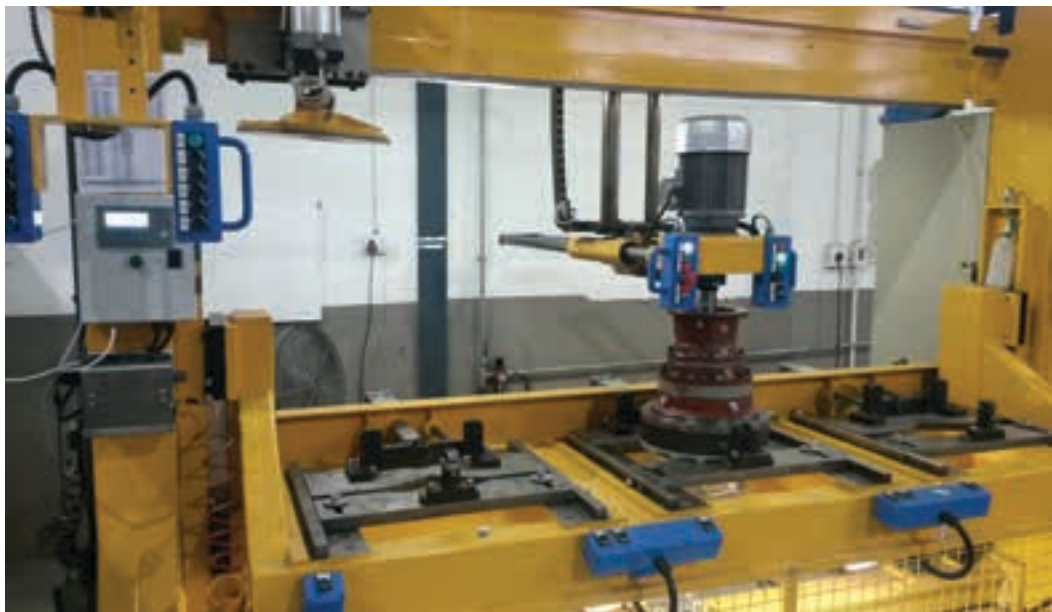
Above: A Bonfiglioli 300-series planetary drive under test at Bonfiglioli’s ISO 9001: 2008 accredited Linbro Park assembly facility.
