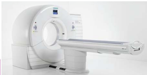
FIG. 1. Technical realization of a DSCT system (SOMATOM Definition, Siemens Healthcare, Forchheim, Germany). One detector (A) covers the entire scan field of view with a diameter of 50 cm, while the other detector (B) is restricted to a smaller, central field of view.
