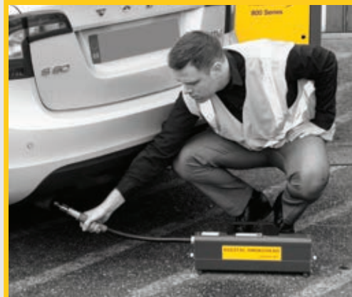
Digital smoke meter with automatic calibration
