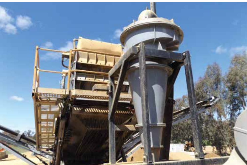
The FM120C is equipped with a single rubber-lined G4 660 hydrocyclone that classifies at 75 microns.
