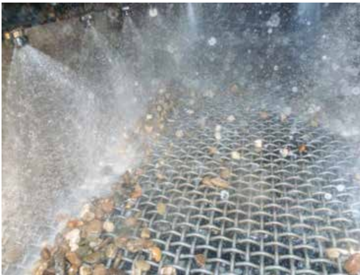
The M1700's three-deck screen features over 140 spray nozzles that give full spray coverage.
