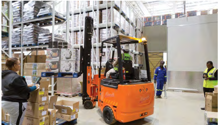
Goscor Lift Truck's Bendi range can work in very narrow aisle width. By decreasing aisle width, most warehouses can save up to 40% of their warehouse space.
