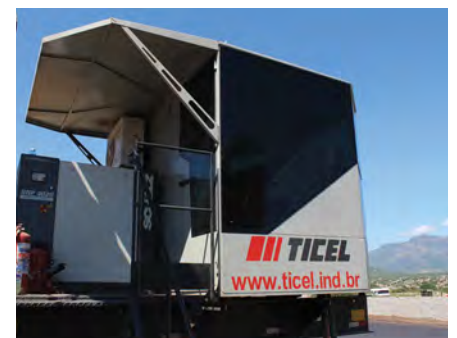
The control cabin allows for remote operation and monitoring of all plant functions through cameras and sensors.
