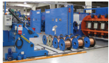
▲ Rigid strander with automatic loading system
